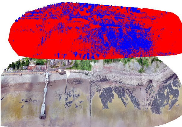
Figure 6 – 2015 DSM with 2016 Orthomosaic. On top is the 2015 DSM showing the areas of cut and fill and the 2016 Orthomosaic below. The red segments on the DSM are the areas of materials loss and the blue segment are the areas of material gains.
