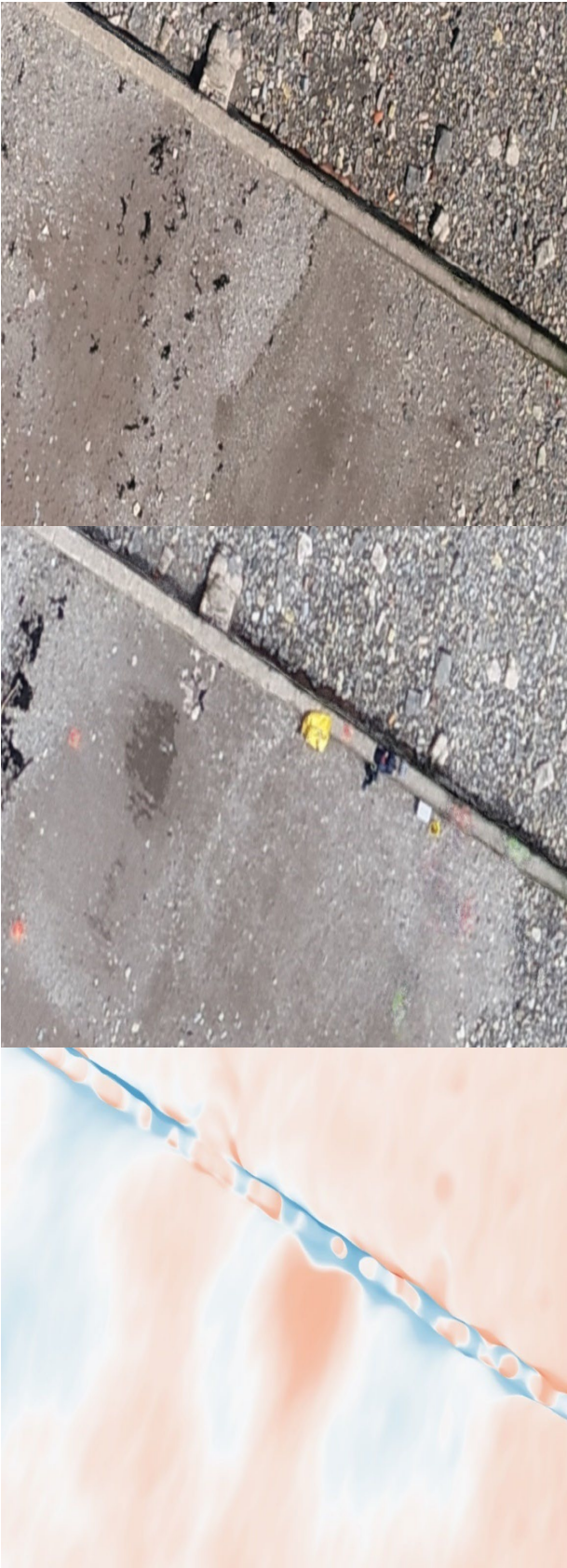
Figure 19 - Close-up View of the Area around the Groyne. (Survey 1, 2 and Difference Map respectively).
