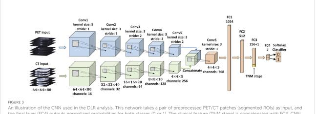
the final layer (FC4) outputs normalized probabilities for both classes (0 or 1). The clinical feature (TNM stage) is concatenated with FC3. CNN, convolutional neural network; DLR, deep learning-based radiomics; ROIs, regions of interest.
