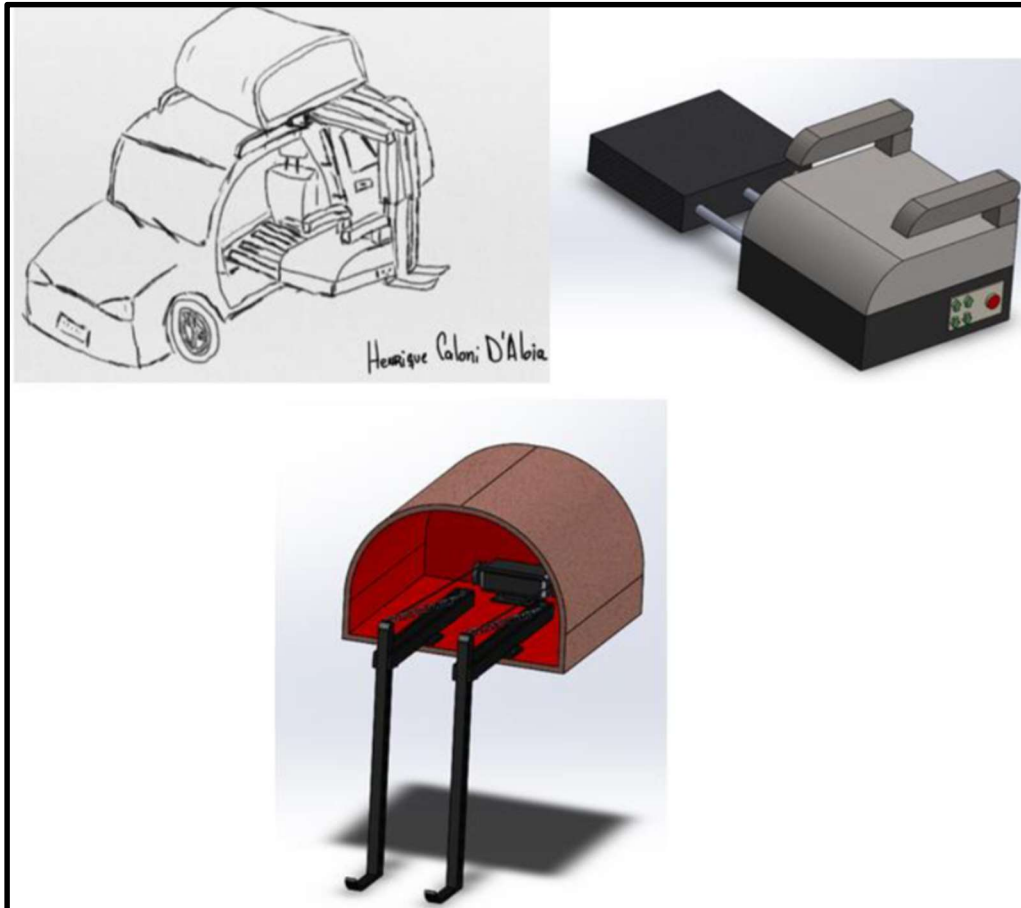
Figure 45- Comparison between initial isometric drawing made by hand and final result in 3D CAD
