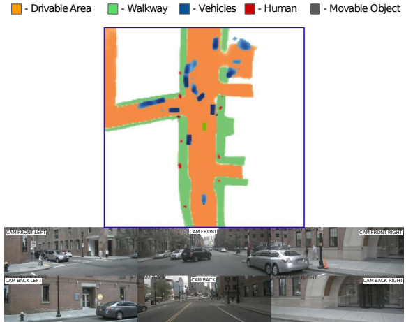
Fig. 1: Semantic grid predictions by LAPNet for classes in the NuScenes dataset [7]. By using LIDAR information to aid the projection of camera features, our method allows the creation of more precise semantic grids compared to camera-only methods. Best viewed with digital zoom.
