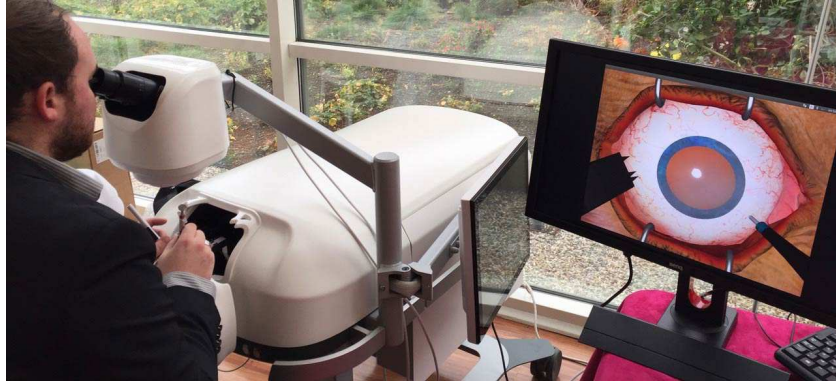
Figure 1.2: Retina surgery simulator with haptic feedback
