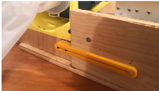
Figure 7: Side adjustable lock (orange color)
