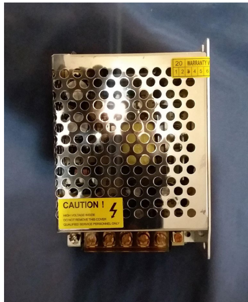
Figure 3: Power supply unit
