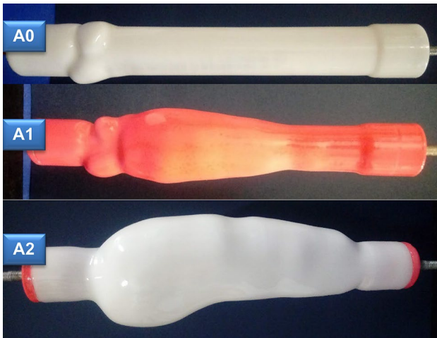
Fig. 1 Moulds used to cast the aortic models. A0 ) Normal aorta; A1 ) 48 mm diameter aorta; A2 ) 64 mm diameter aorta
