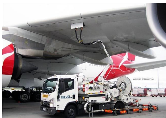
Figure 1.6. Hydrant dispenser refuelling vehicle [9]
