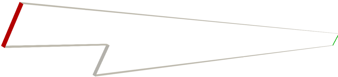
Figure 3.10: Boundary conditions applied to the problem of the Backward facing step, inlet (red), outlet (green), and fixed walls (grey)
