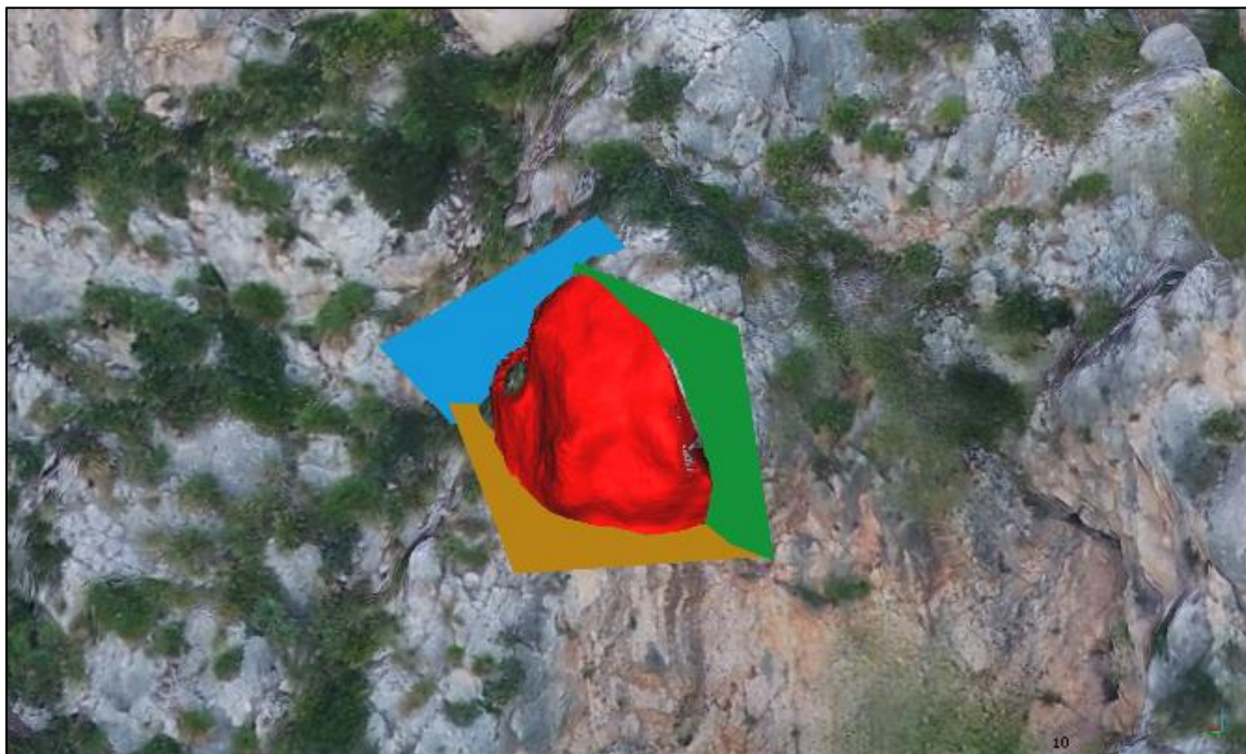
Fig. 4 Example of a potentially unstable block identified using the joint pattern characterized in the point cloud and extrapolated to cut the 3D mesh.
