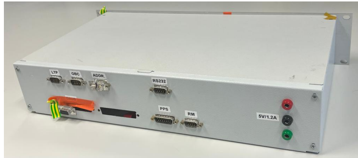
Figure 3.7: Container used to keep the temperature fluctuations inside.
