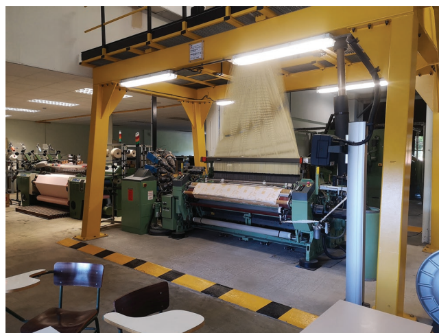
Figure 2. Dornier LWV8/J weaving machine moved by a Jacquard Stäubli LX1600B.
