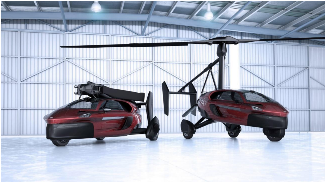
Figure 3.8. Pal-V Pioneer flying car in both ground and flight driving modes [14].
