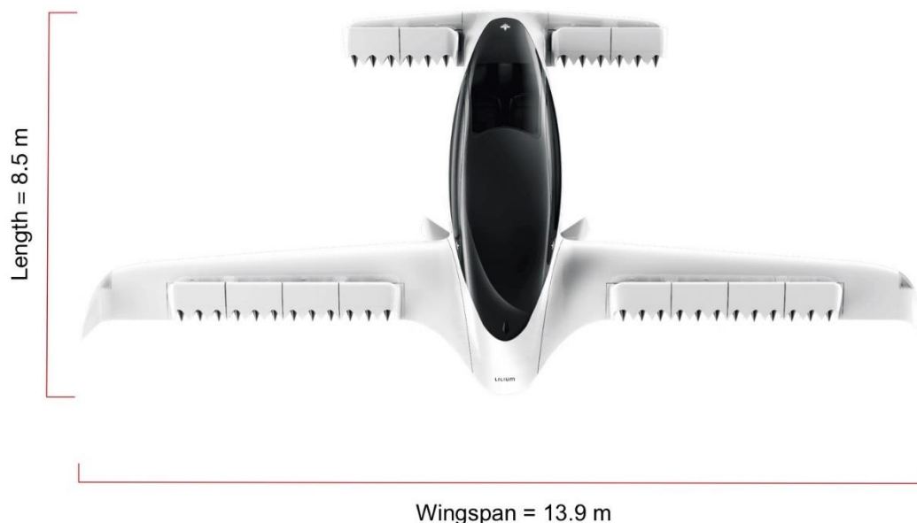
Figure 6.3. Lilium JET by Lilium main dimensions (scheme done by own elaboration based on [25]).
