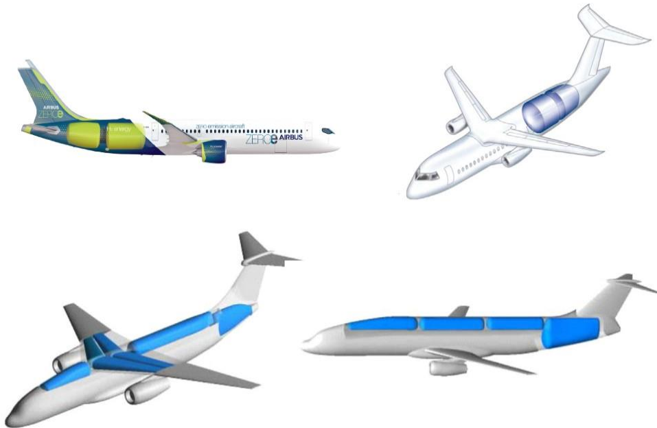
Fig. 3.21 Possible integral tanks designs [9]
