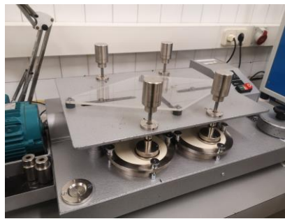
Figure 2. Martindale machine performing a test.
