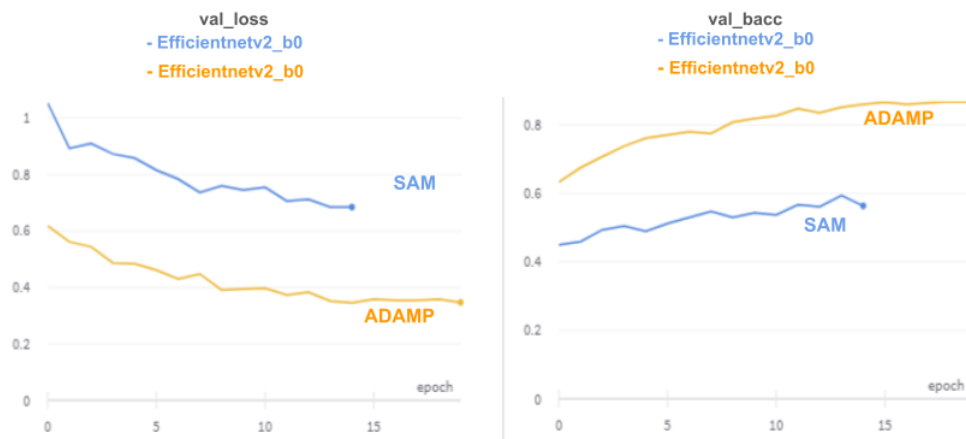
Figure 6.2: Run comparison of SAM and AdamP on the rapid and low parameter EfficientNetV2-B0. The tendency shows that SAM requires almost twice the time to reach comparable results to AdamP.
