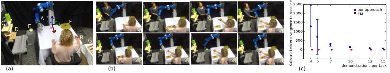
Fig. 5. (a) We evaluate our approach in a collaborative scenario where a robot (A) assists a human (B) in making a salad. Hereby the robot can hand over the board (D) the dressing (C), a tomato (F), the bowl (E) or assist with a standup motion. (b) The demonstrations are recorded as human and robot trajectories where the robot is moved in kinesthetic teaching mode and the wrist trajectory is tracked with a motion capturing system. (c) We again compare the KL-divergence of both our approach and an EM approach to a baseline from labeled data. For an increasing number of demonstrations per task our approach converges to the EM solution but requires less recomputation and memory as new demonstrations arrive.
