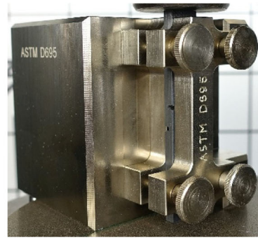
Figure 5. Compression shear test according to ASTM D 3846: (left) specimen geometry and (right) experimental setup.
