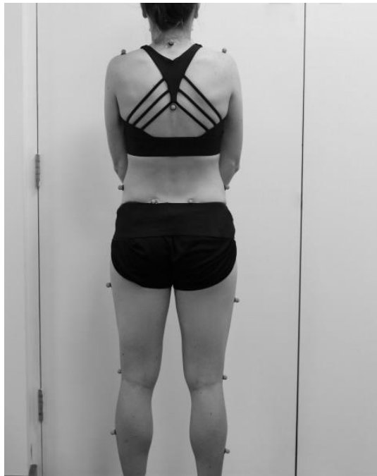
Figure 17 Posterior view of experimental set up for motion analysis demonstrating attachment sites of the Vicon reflective markers and inertial measurement units.
