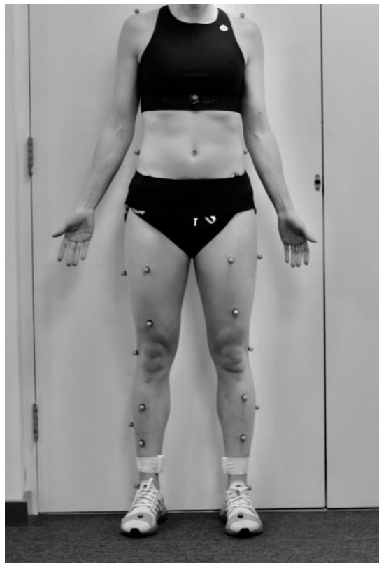
Figure 18 Anterior view of experimental set up for motion analysis demonstrating attachment sites of the Vicon reflective markers and inertial measurement units.
