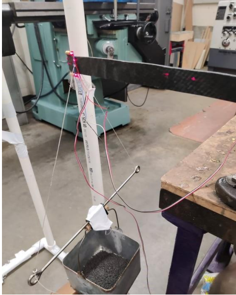
Fig 3. 7. Nylon string used to hold loading bucket
