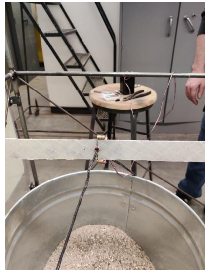
Fig. 4. 4. Laser dots mounted for deformation
