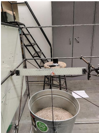
Fig. 4. 3. Beams screwed for boundary condition
