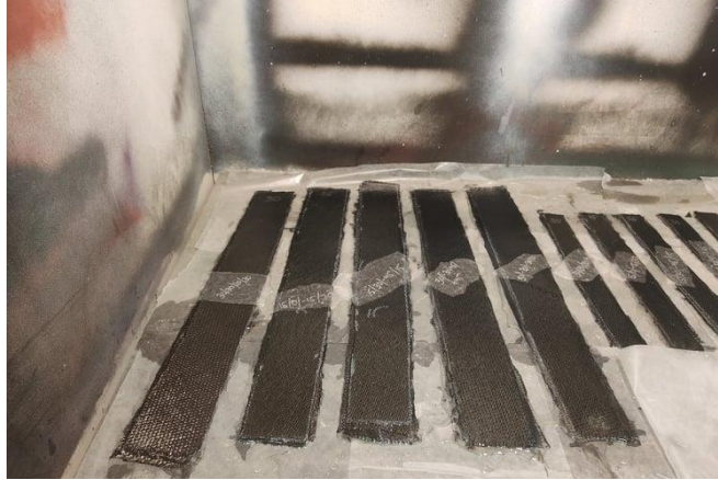
Fig 3. 2. Beams left for curing after fabrication
