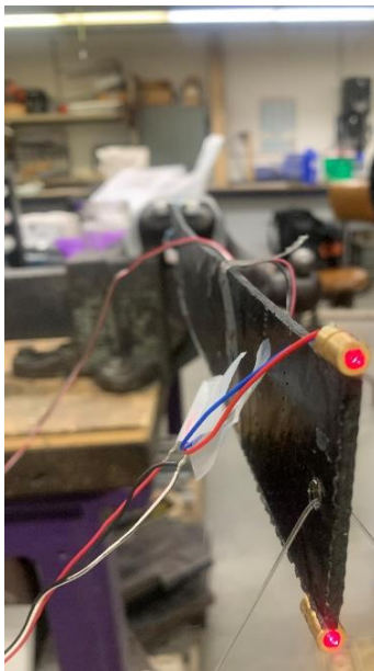
Fig 3. 5. Mounting laser dots for tracing the angle of twist.
