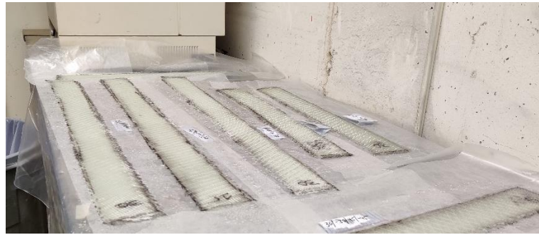
Fig. 4.1. Beams left for curing at room temperature
