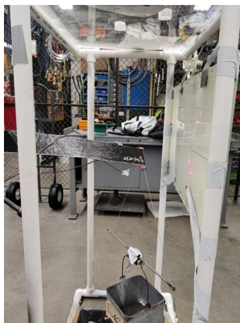
Fig 3. 6. Beam in buckling configuration with laser dots reflected on the tracing screen.
