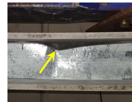
Fig. 7. Test results for Z02 specimen: (a) moment-displacement plot; (b) buckling curve obtained from CUFSM; and (c–f) failure modes of the sheathing-fastener connections.
