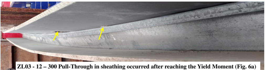
Fig. 8. Test results for ZL03 specimen: (a) moment-displacement plot; (b) buckling curve obtained from CUFMS; and (c–f) failure modes of the sheathing-fastener connections.
