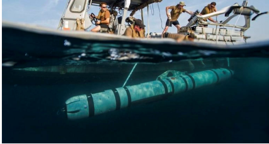
Figure 15. A Mk 18 Mod 2 Kingfish. Source: Gain (2019).
