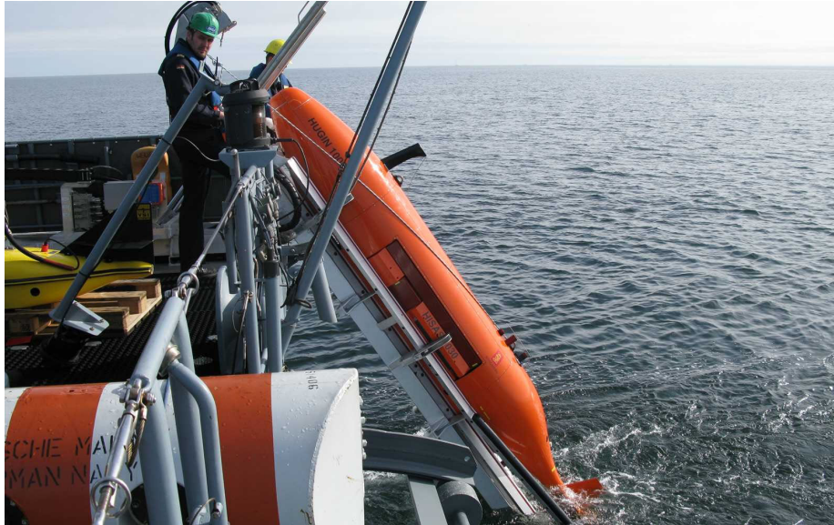
Figure 16. AUV Hugin. Source: Kongsberg (n.d.).
