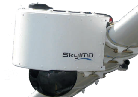
Figure 37. TASE 200 sensor in SkyIMD enclosure
