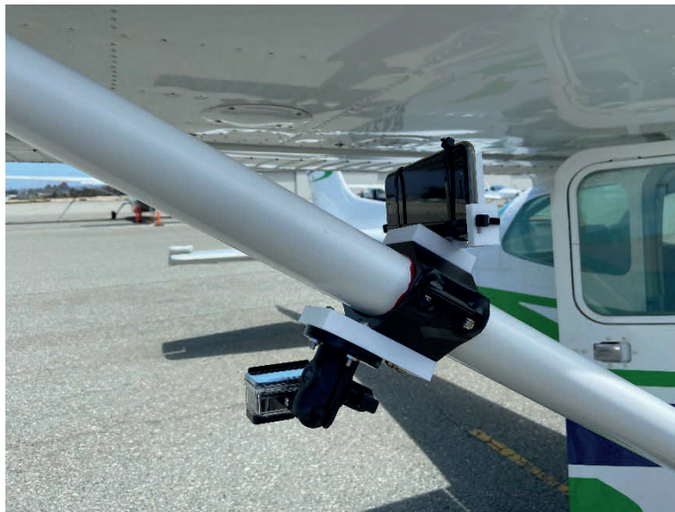
Figure 54. Mounting setup of acquisition equipment on Cessna wing strut
