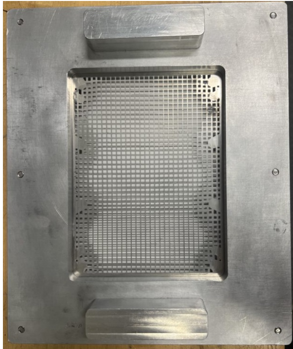
Figure 4.9. Thermal Grease Stencil - Front View for Aligning IGBT Module
