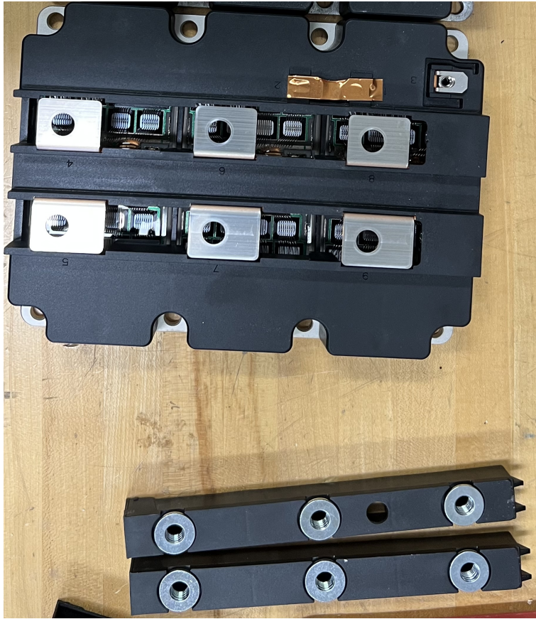
Figure 4.2. IGBT Module with Modified Bus Bar Connection Plate
