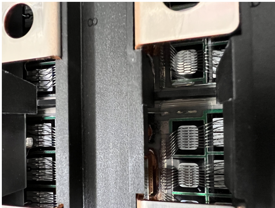
Figure 4.4. IGBT Module Chip Closeup
