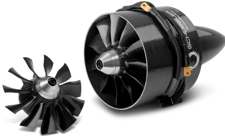
Figure 2. Advanced single stage EDF design. Source: [3].
