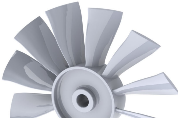
Figure 32. Final CAD model of the fan rotor.
