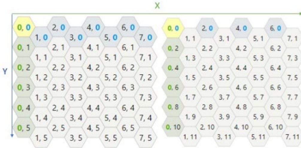
Figure 11. Hexagonal boards left without double coordinates and right with double coordinates. Source: [10].
