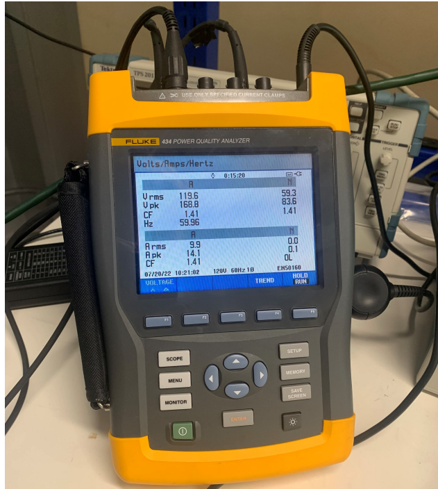
Figure 3.15. The Fluke 434 Power Quality Analyzer measurement instrument is used to monitor and capture voltage, current, power and frequency information, among other characteristic parameters.
