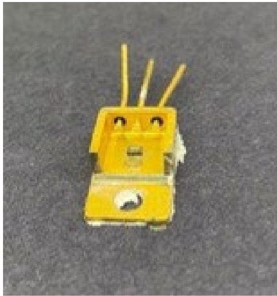
Figure 26. Image of Commercial Device with Sidewall Cut away to Allow Positioning Fiber Cable to Couple Light from the Die
