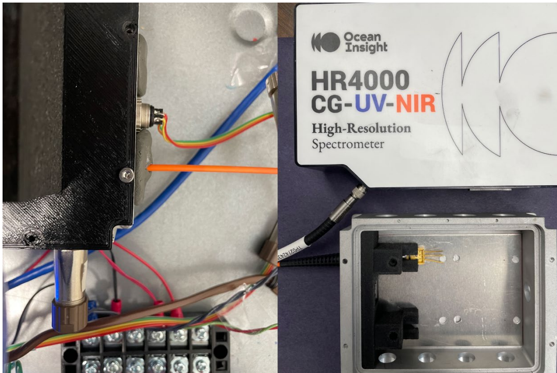
Figure 11. Fiber Cable and DUT Chamber with PLA Lid Installed (left), Prototyping of Spectrometer Integration to DUT Chamber with Device Installed in Cradle (right)
