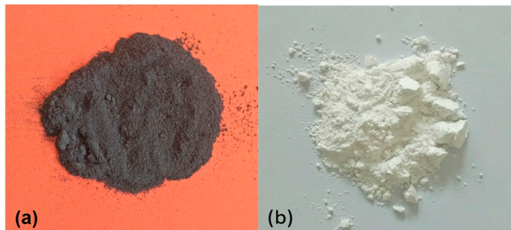
Figure 5. Sample photographs of: (a) Graphene nanoplatelets; (b) MgO NPs.
