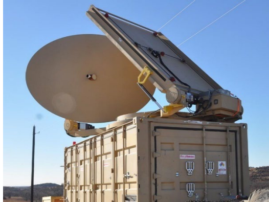
Figure 22. Phaser HPM system. Source: Raytheon Technologies (2020).
