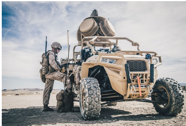
Figure 13. LMADIS mounted on Polaris MRZR Marine vehicle. Source: Liptak (2019).
