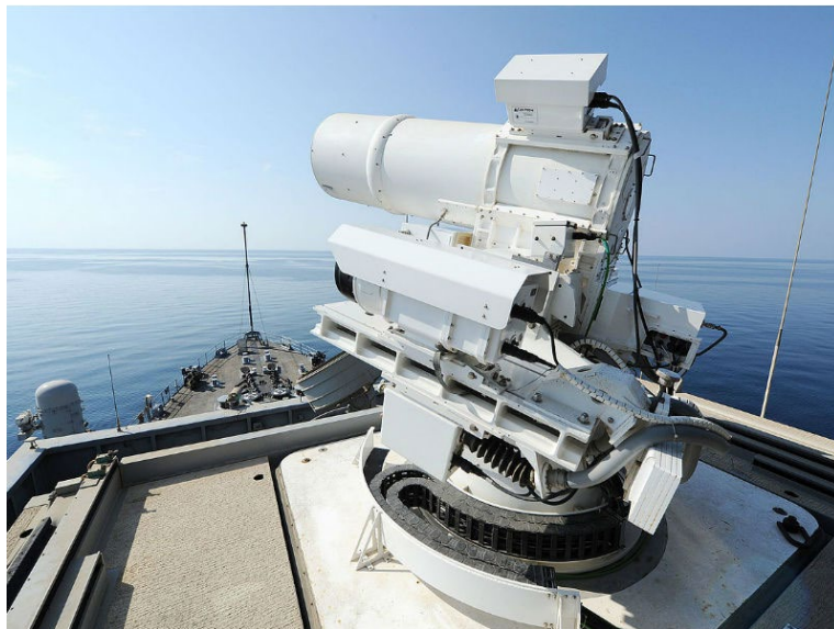
Figure 21. HELIOS, a Navy laser weapons system in development. Source: Hussein (2019).
