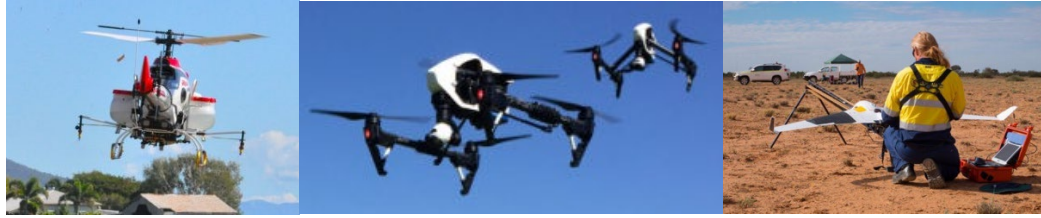
Figure 4. Multirotor, fixed wing and single rotor UAS. Source: Chapman (2019).
