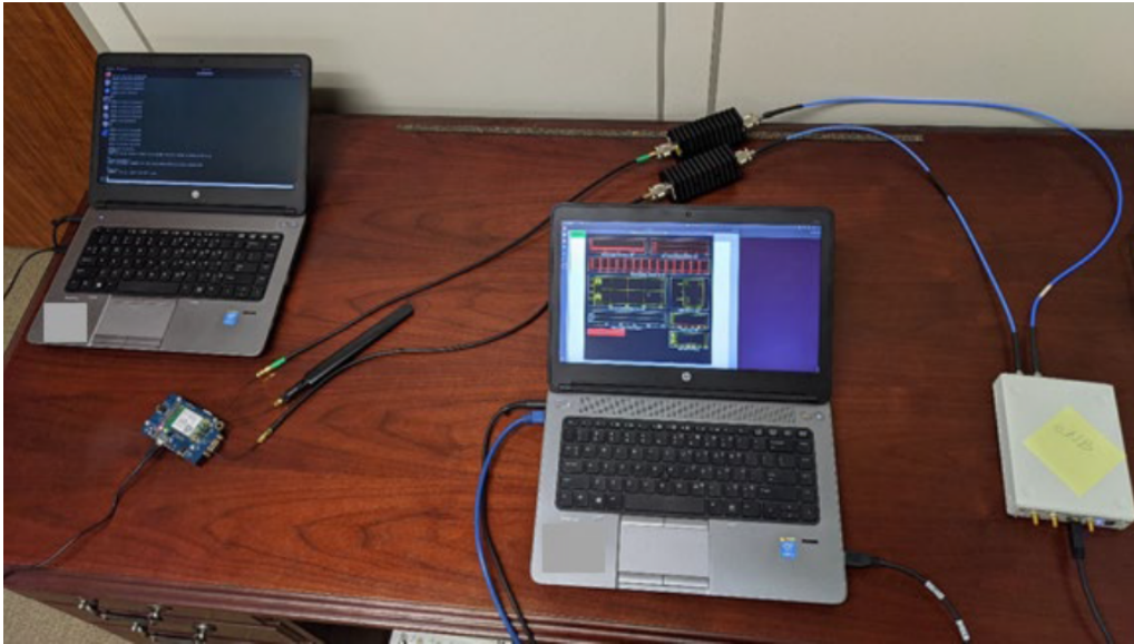
Figure 3.6. Previous Wired 4G LTE Open Stack Network with Simulated UE and Attenuators. Source: [11]
