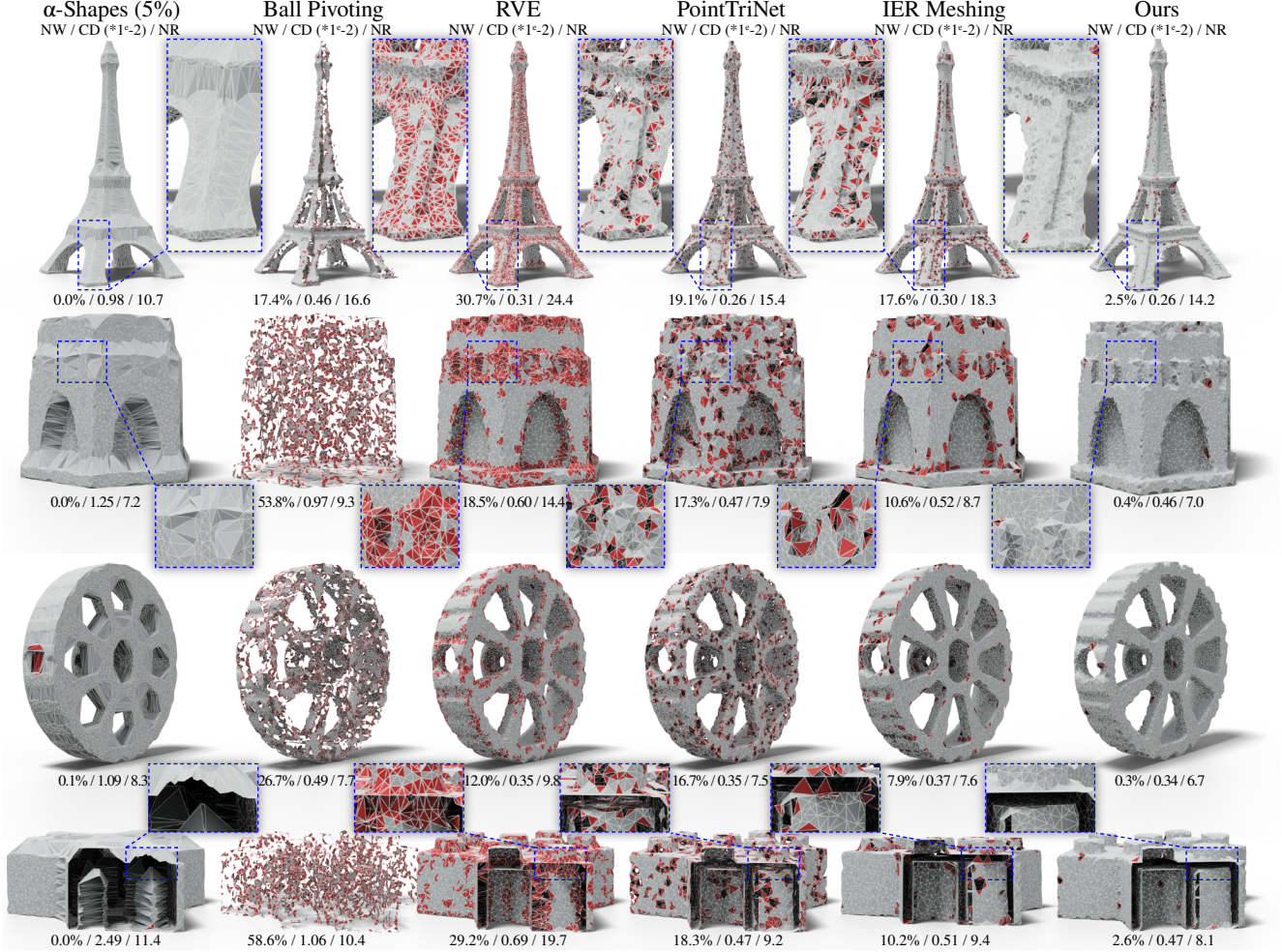
Figure 5. Qualitative comparison. We compare four meshes reconstructed by our method to the results of five current methods. Non-manifold triangles are marked in red and we show both the percentage of non-watertight edges (NW) and the Chamfer distance multiplied by 100 (CD) below each shape. Note that classical non-data-driven methods struggle to separate thin surfaces and data-driven methods have significantly more non-manifold triangles.
