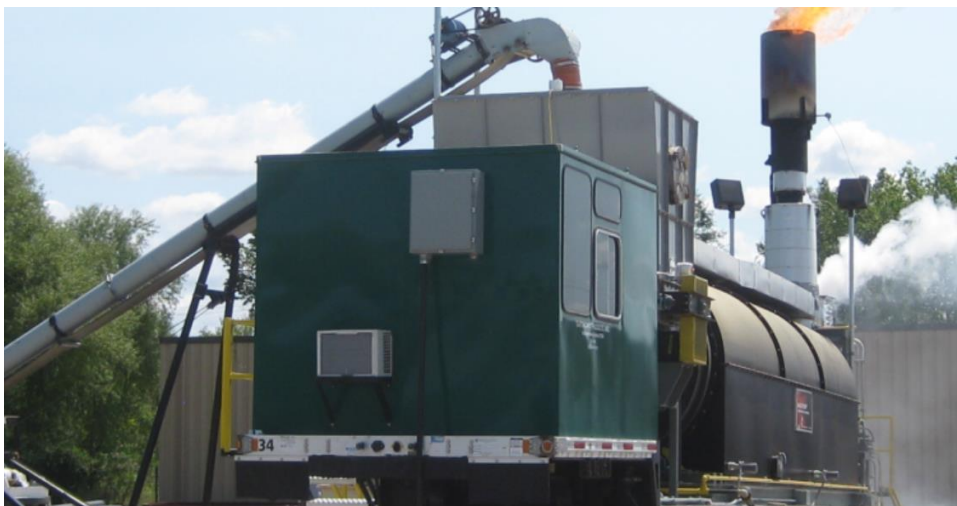
Figure 24. The mobile torrefaction system in operation [89].
