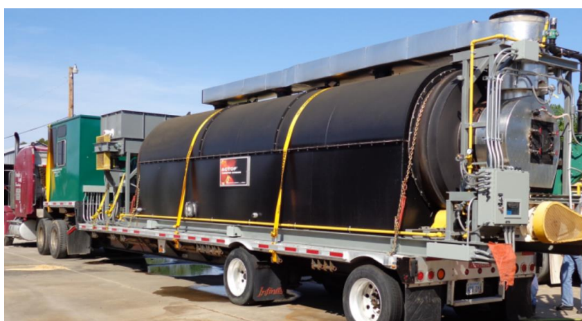
Figure 25. The mobile torrefaction system is in a package and ready to move [89].
