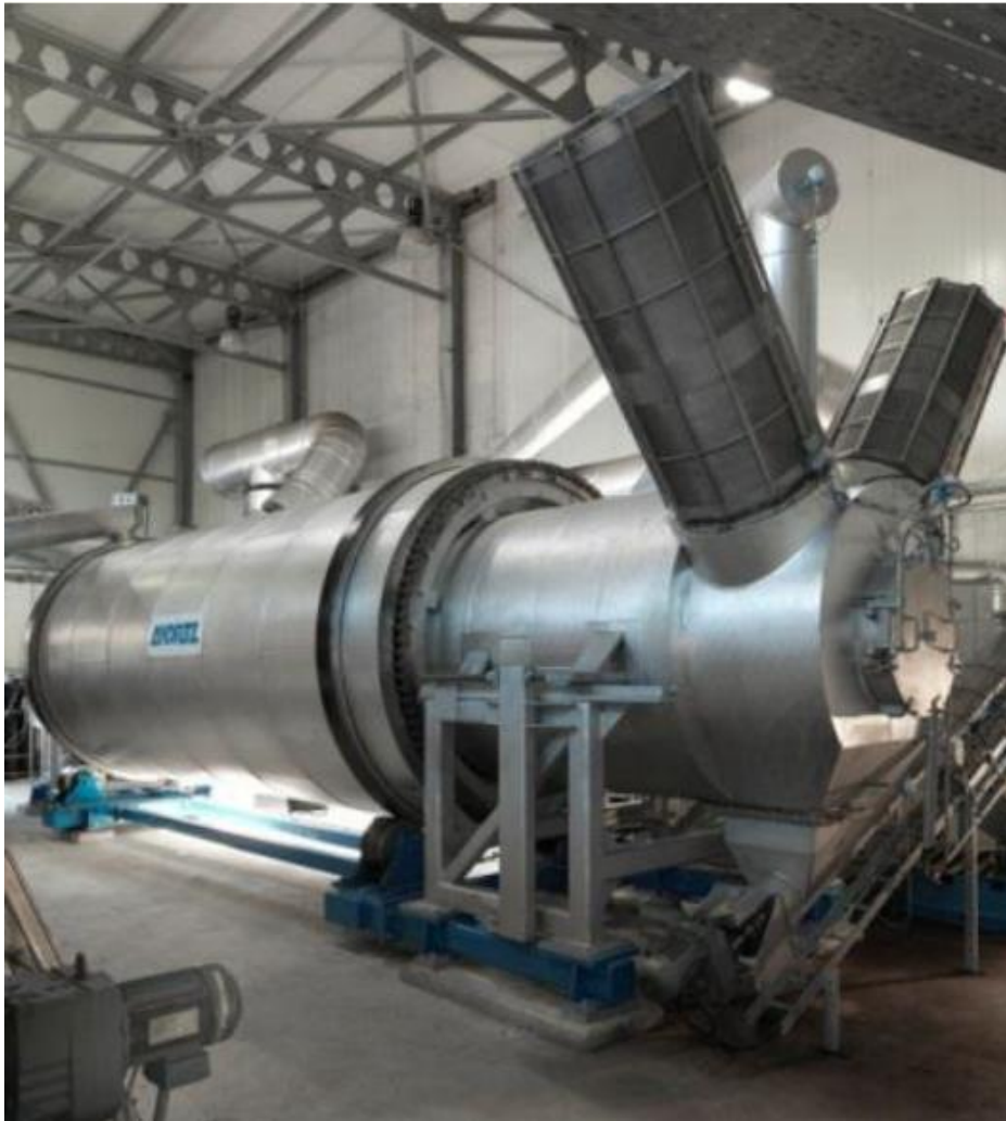
Figure 12. A commercial scale rotary drum reactor for biomass torrefaction [44].
