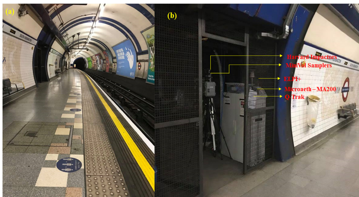
Fig. 1. (a) South Kensington Underground Station, Piccadilly line eastbound platform #4. (b) Air sampling equipment was placed on the station platform.
