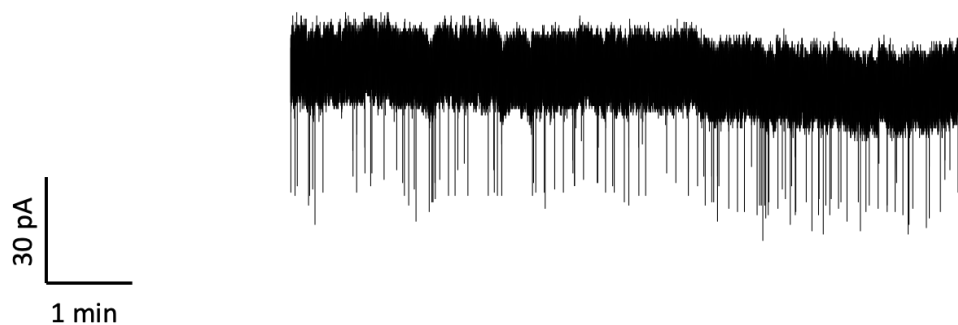
Figure 2.7: Sample current trace for cis-to-trans with 10 Kbp DNA. DNA concentration is 100 pM and the experimental conditions are a 30 KHz low-pass Bessel filter, 100 KHz sampling rate, 100 mM KCl in TE pH 8.0, and -300 mV. The peak amplitude is typically around 30 pA, and so has good SNR compared to the baseline.
