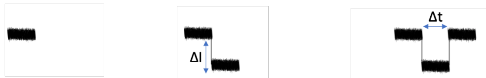
Figure 2.5: Schematic of the DNA moving through the pore in the nanopore experimental setup and the subsequent current changes when the DNA moves through the pore. The time the current is changed is called the dwell time and how much the current is affected is called the peak amplitude. After the DNA moves through the pore, the current returns to its baseline.
