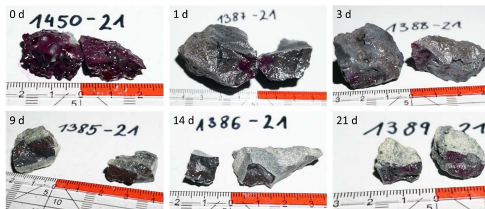
Figure 20. Determination of the carbonation depth using phenolphthalein.
