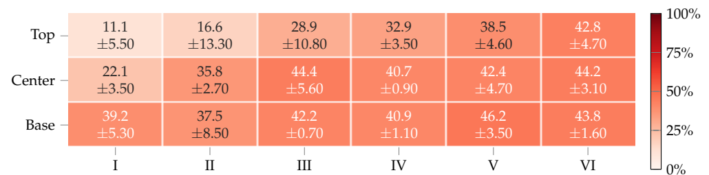
Figure 10. Average FVC and standard deviations of three different samples molded with process Configuration B are analyzed via thermal gravimetric analysis. The partitioning follows the illustration in Figure 1b, where the red dotted lines indicate the separation between top, center and base of the coupons.
