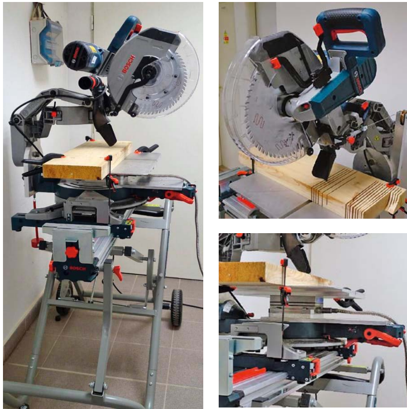
Figure 2 View of Bosch mitre saw test device with Kistler dynamometer Slika 2. Pogled na poprečnu klatnu pilu Bosch s Kistlerovim dinamometrom
