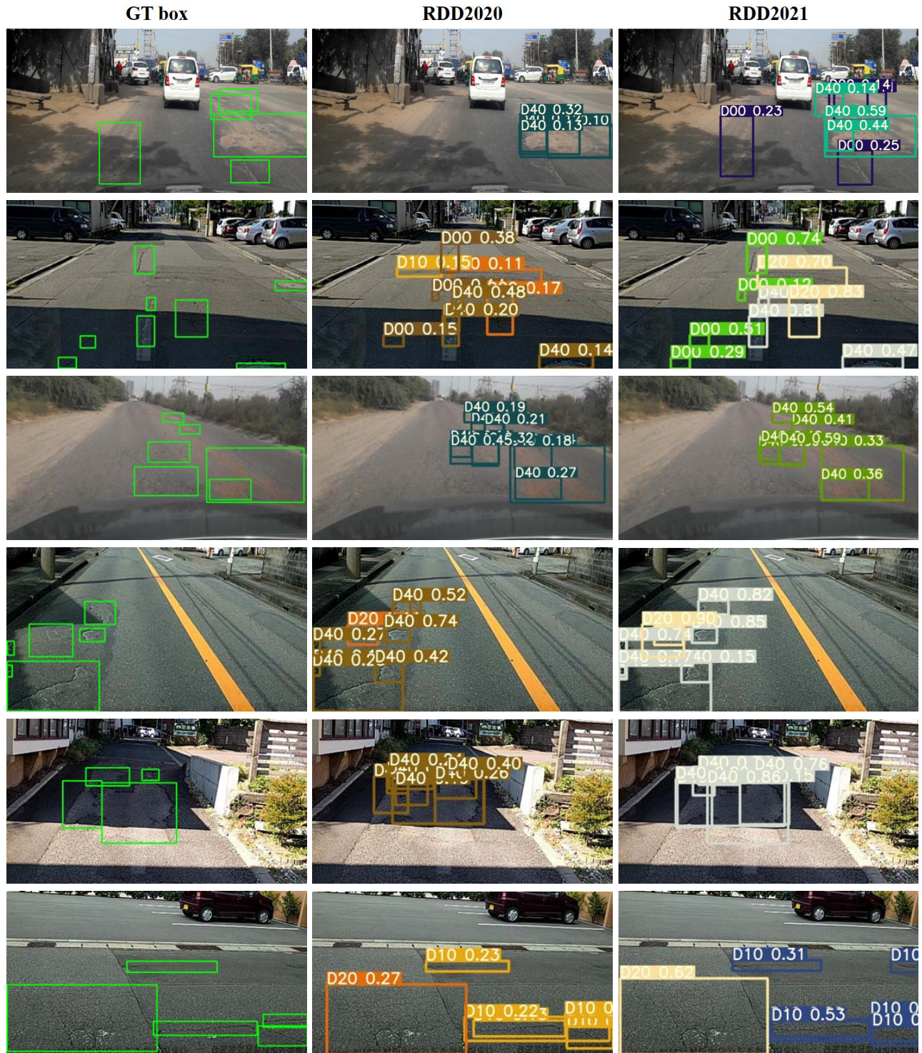
Fig. 7. Visualizations on RDD2020 and RDD2021, respectively. For each row, we present the Ground-Truth box (GT box), the predicted boxes on RDD2020 and RDD2021 achieved by YOLOv5 [19] and Faster RCNN [12]. Obviously, the model suffers from low-confidence predictions or false negatives due to the scarce of sample on RDD2020, while RDD2021 provides a large amount of damage types and appearances, facilitating the more accurate and robust detection performance. Best viewed in color.
