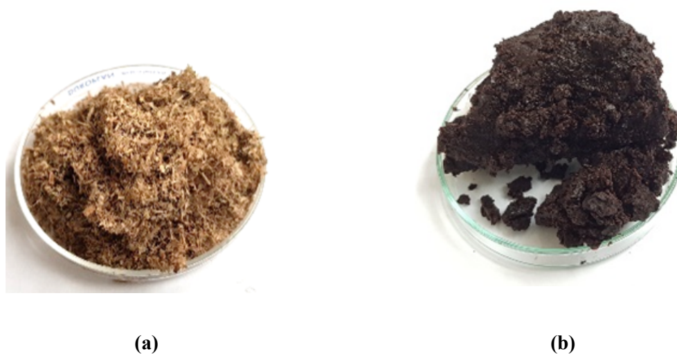
Figure 1. (a) dried and ground water hyacinth material; (b) dewatered alum sludge cake sample collected from a treatment plant of Scottish Water.
