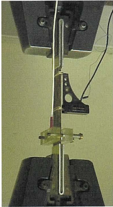
Plate 6.2 Photos of acoustic emissions analysis tensile test set-up.
