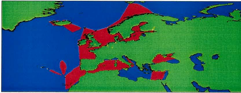
Fig. 10: Red highlights the region in which it pays to use RAAS: ie we are within a triangle of three stations, each of which meets full coverage criteria by day.
