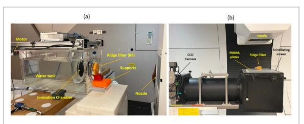
$\textbf{Figure 3.} \ \text{Experimental setup: (a) range scanner with RF placed closed to the isocenter, (b) CCD camera with PMMA plates and RF. \\$
