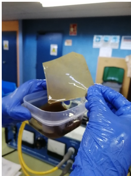
Figure 6.1. Samples tested in the AC and impulse BDV tests
