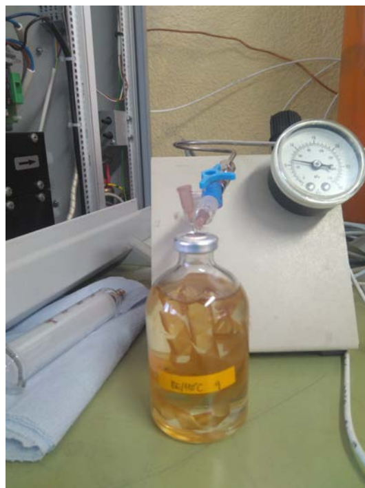
Figure 7.2. Bubbling treatment with nitrogen.
