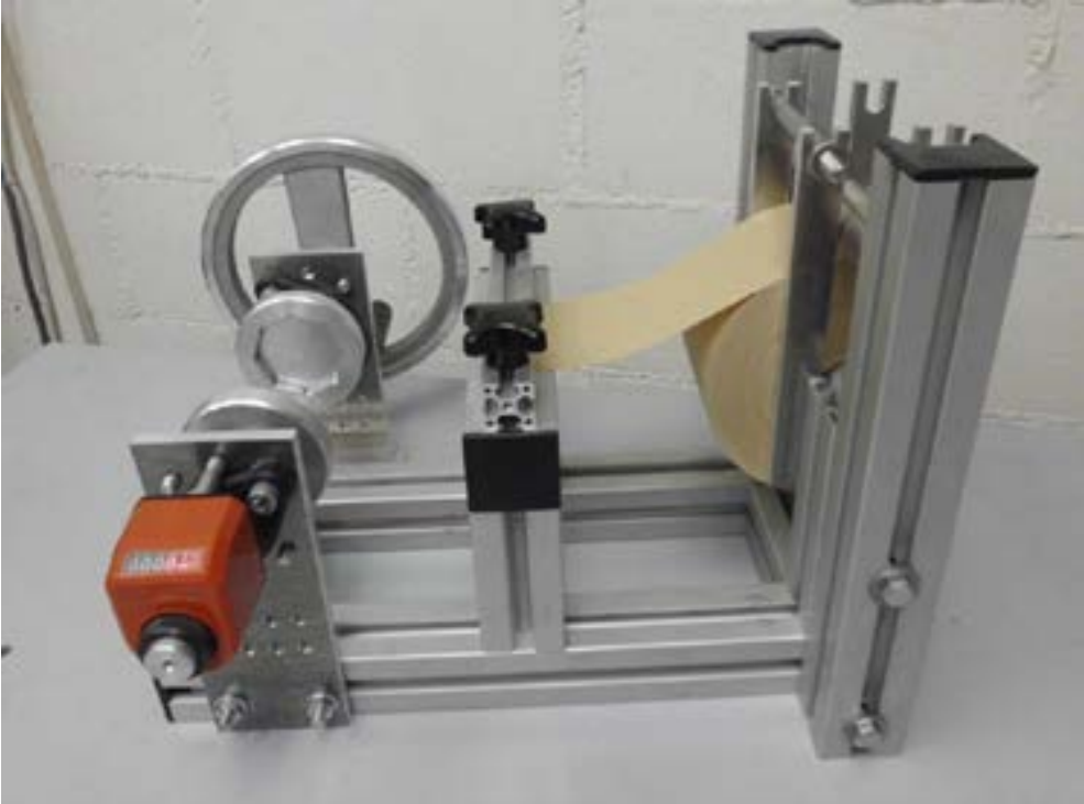
Figure 5.3. Winder machine deployed to prepare the solid insulation test-specimens
