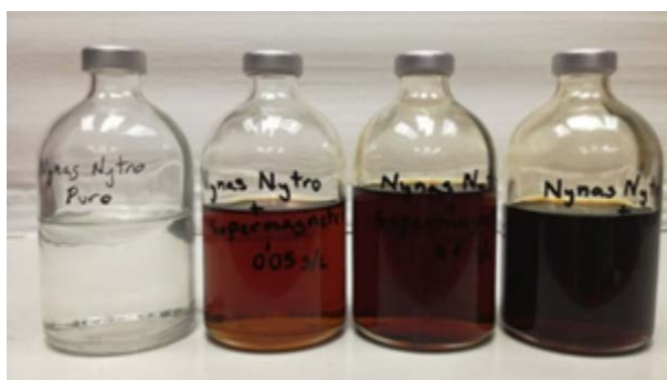
Figure 3.5. NFs prepared from the MO Nytro 4000x with several NP concentrations.
