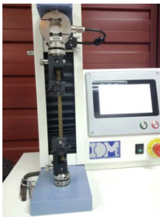
Figure 7.4. MTC-100 Vertical Universal Tensile Tester (IDM)
