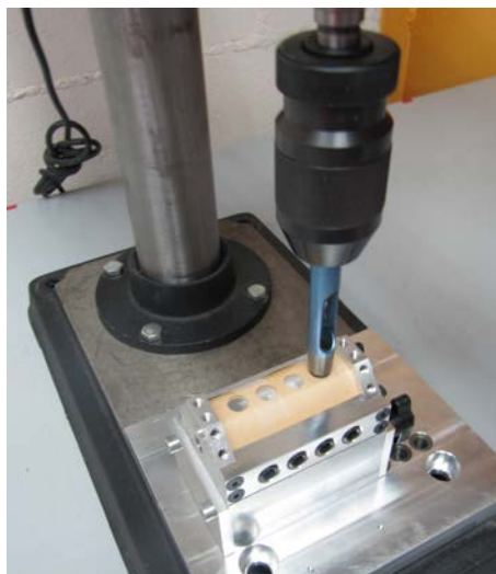
Figure 4.2. Extraction of samples from the paper coil
