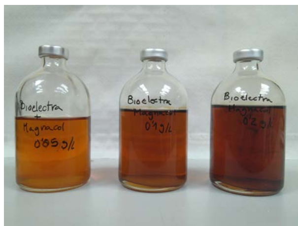
Figure 3.4. NFs prepared from the NE Bioelectra with several NP concentrations.
