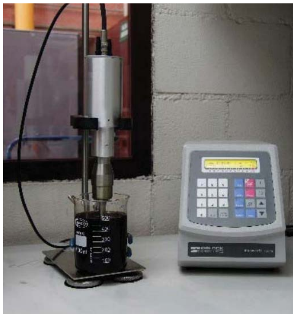
Figure 3.3. Ultrasounds stirrer used to produce the NFs through the Thesis.
