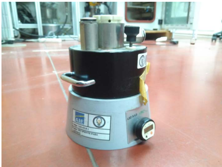
Figure 5.2. Liquids' test cell
