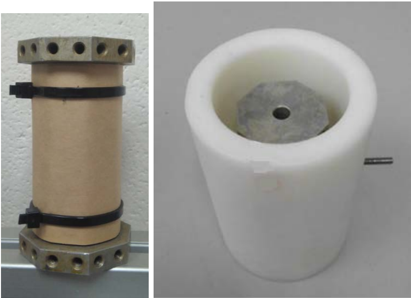
Figure 5.4. Cellulose test specimen and test cell
