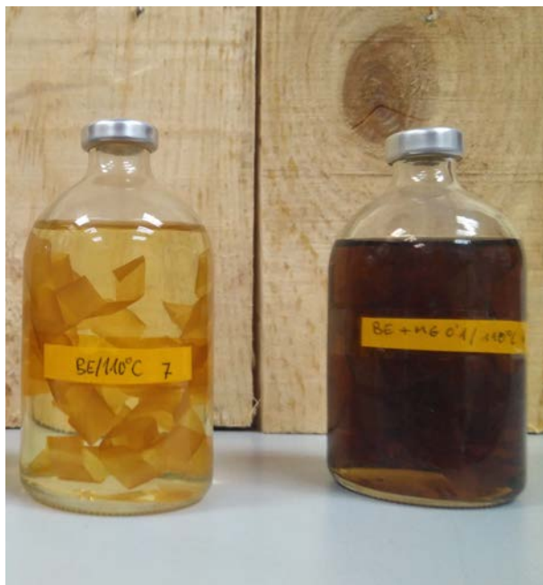
Figure 7.1. NF and NE aging test vials.
