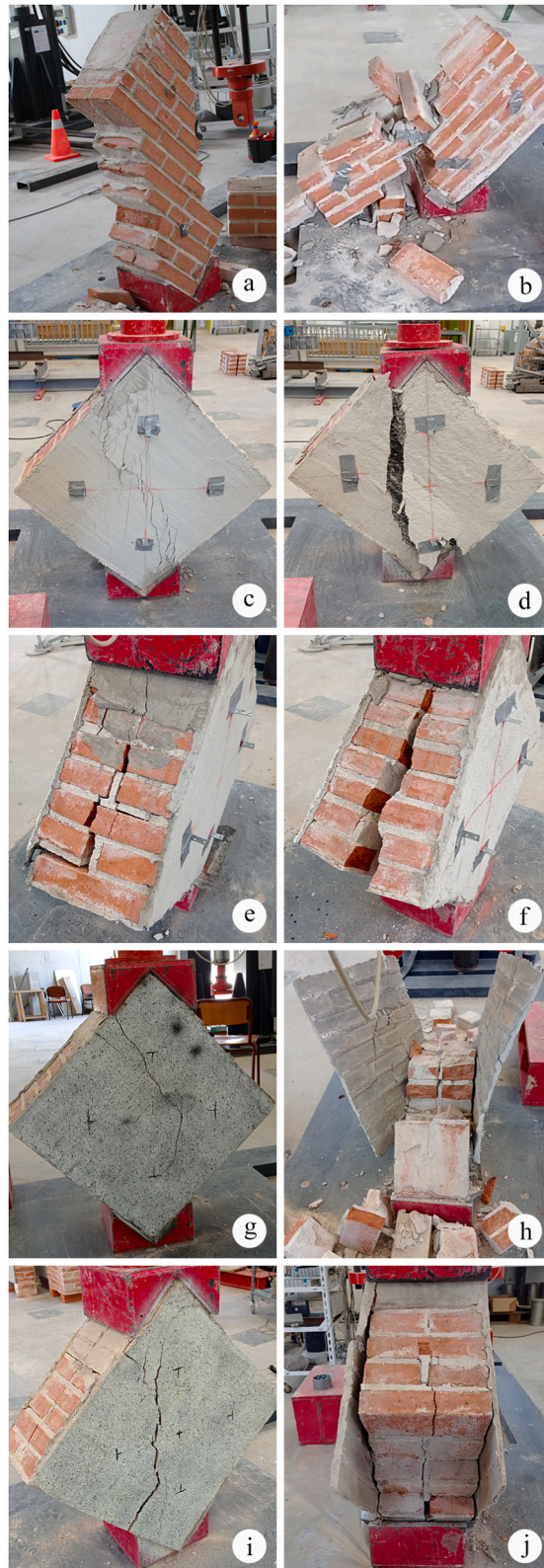
Fig. 7. Examples of failure modes in the different series tested: (a) N20; (b) N600; (c) G20; (d) C20; (e) G600a; (f) C600a; (g-h) G600b; (i-j) C600b.
