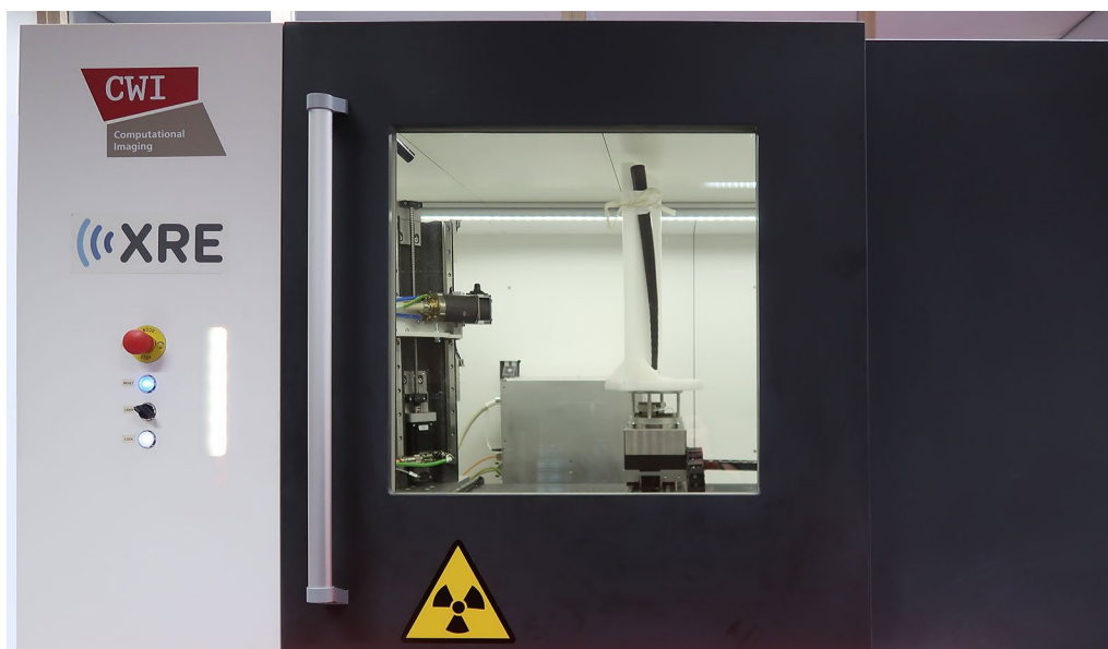
Fig. 4 Set-up of CT scanning the cornett at the CWI, cornett BK-AM-62-B mounted on a custom made Ethafoam ® stand
