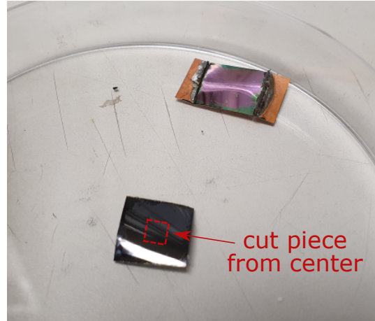
FIGURE 6.1: Bottom part: Exfoliated 12\text{ mm} \times 12\text{ mm} REBCO sample, which was soldered on a brass block, stripped off the metallic substrate and removed from the block again by melting the solder. We cut out a \approx 3.5\text{ mm} \times 3.5\text{ mm} piece from the center (red dashed square) and measured its magnetization. Top part: The complementary substrate side CC piece of the exfoliated REBCO sample.
