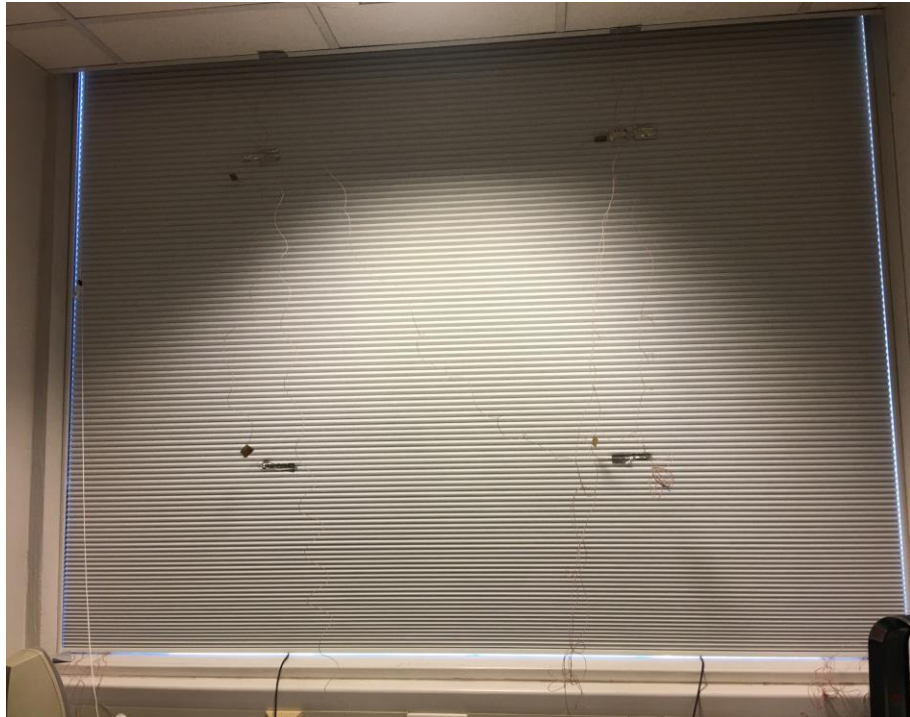
Figure 53: Location of four thermocouples attached to the internal surface of the blind to measure blind surface temperature
