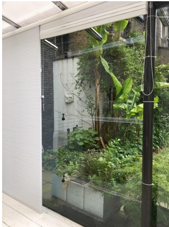
Figure 35: Thermocouples on the glass, globe sensors between blind and glass
