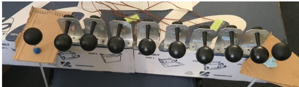
Figure 37: Position of globe sensors during the calibration process
