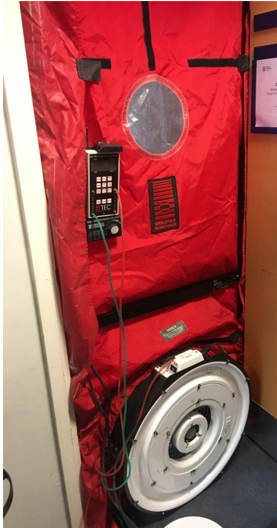
Figure 51: Full blower door equipment viewed from inside including blower door frame, fan and controller with pressure tubes. This equipment was connected to a laptop which is not in the photo.
