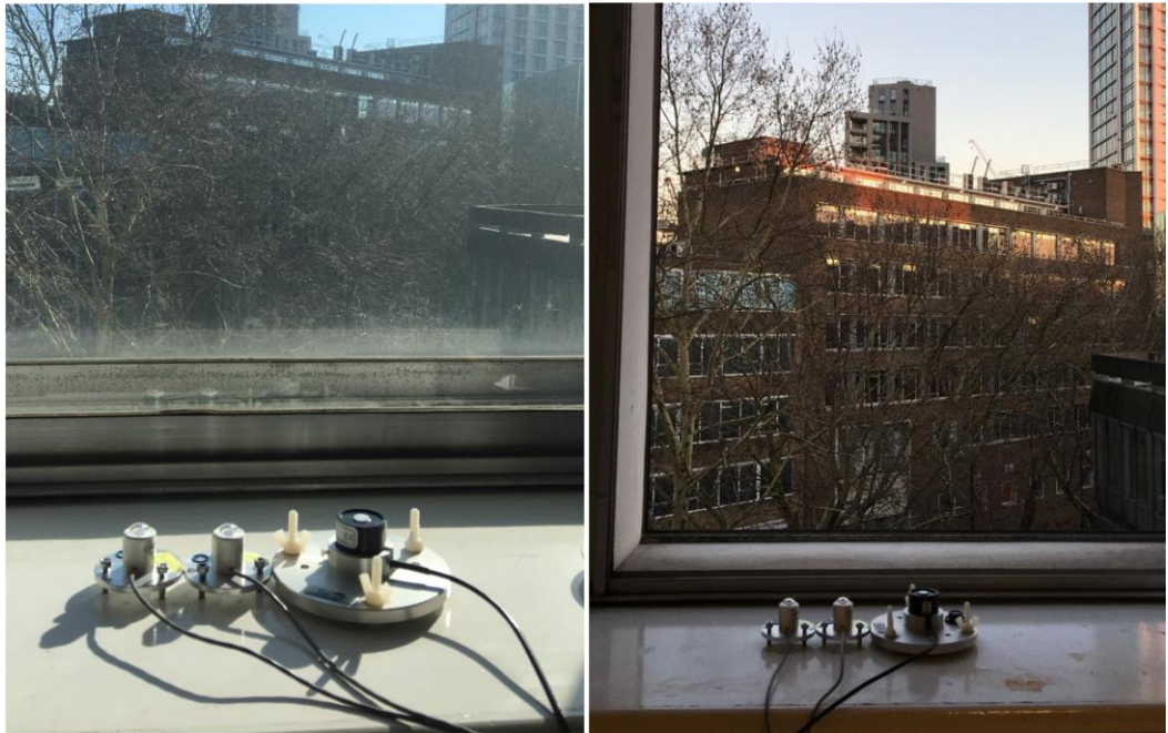
Figure 40: Illuminance sensor calibration at various lux levels
