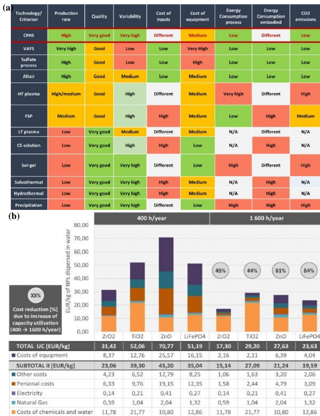
Figure 1.13: (a) Continuous hydrothermal flow synthesis method versus traditional synthetic methods comparison matrix and (b) the cost evaluation table at industrial scale for different nanomaterials produced via CHFS method 300 . Reproduced with permission from reference 300. Copyright 2019 Elsevier.
