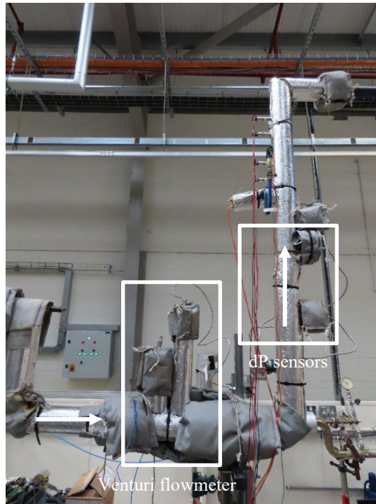
Fig. 3. Test setup side view. Venturi meter is located in the middle and vertical differential pressure section is located on the right.
